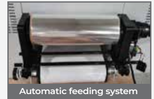
Automatic feeding system
